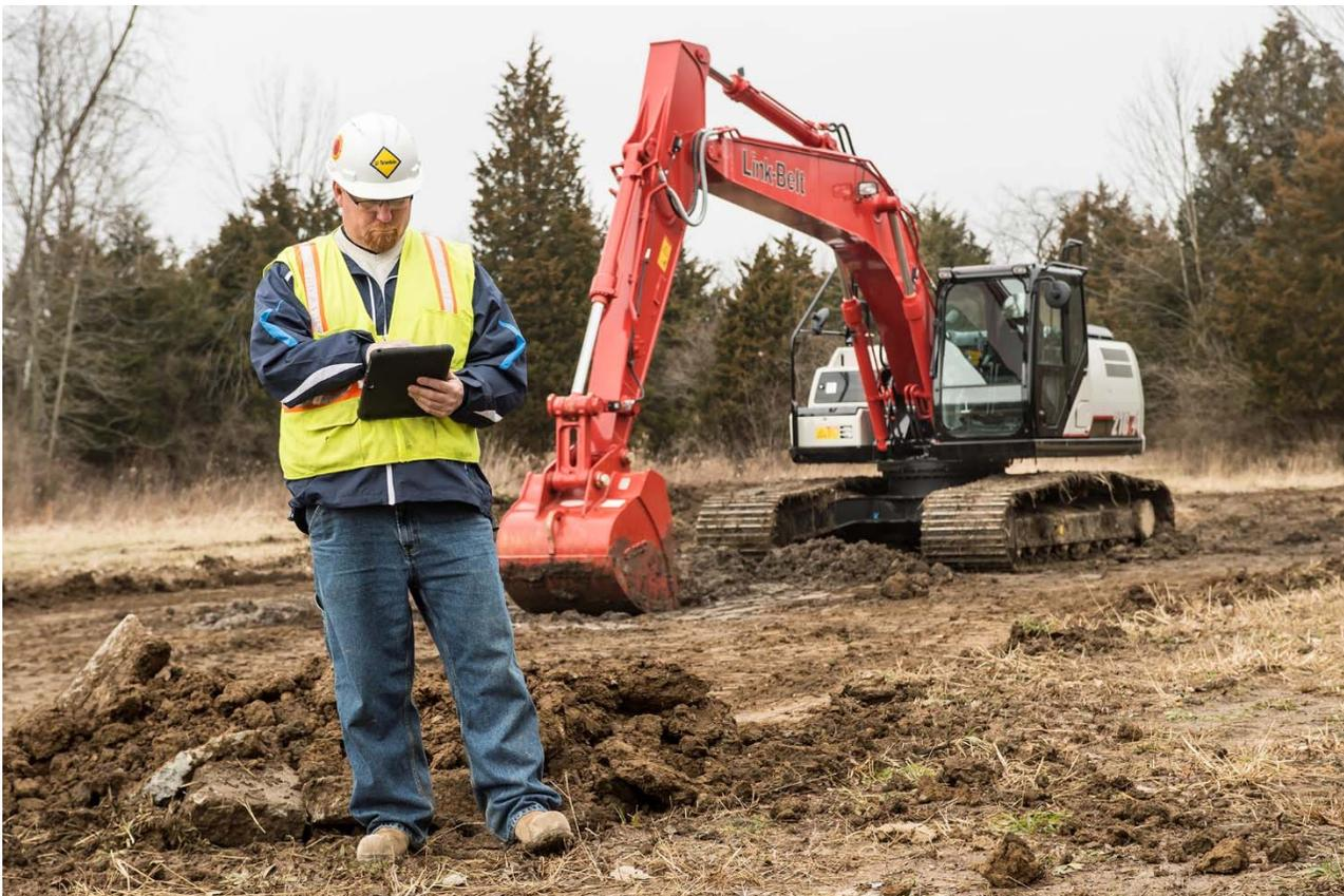
“The 2D Machine Guidance (MG) system can help improve excavator operations on projects such as trenching for underground utilities and pipelines, digging footers and basements, site prep, building roads and mass excavation,” said Adam Woods, LBX Product Manager. “Simply input the target depth, cross slope, and or mainfall slope required from the job and the system will provide visual and audible indication to help the operator maintain a desired grade thus eliminating under or over excavating.”
