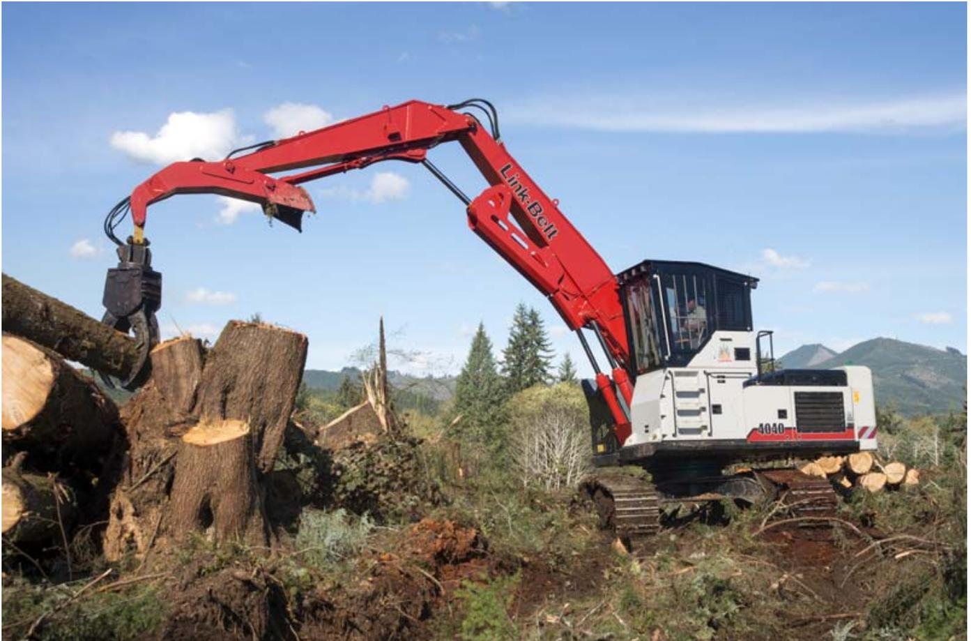
The Link-Belt 4040 TL Forestry Machine is now available for the US and for Canada, with an option for High-Wide or High-Narrow undercarriages to meet transport requirements. Models can be equipped with Live-Heel or Butt-N-Top attachments for log-loading applications. Designed specifically for the 4040 TL, both side- and rear-entry Oregon OSHA/ROPS/WCB certified forestry cabs are available from the factory, with sky roof and escape hatch.
